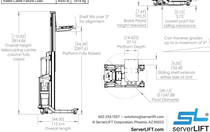
[52.95] 1345.01 Platform height, start of second lift stage (telescoping)
