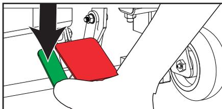
Press on green release pedal until unlocked and slowly pull foot back allowing both pedals to fully retract.
