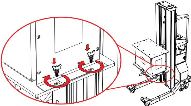
➤ **Note:** Platform Riser should be removed and set aside when not in use. Four holes on Platform Riser top plate are provided for convenient storage of Thumbscrews and Washers when not in use.
