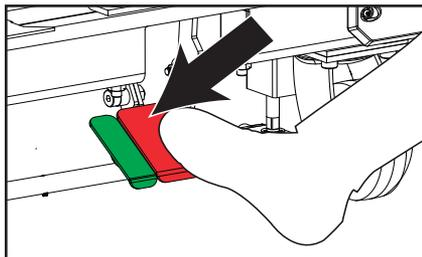
To engage Stabilizer Brake, depress red pedal until it locks in **DOWN** position. The back of the ServerLIFT unit should slightly lift up off the ground. The ServerLIFT unit should not move. If ServerLIFT unit moves, the Stabilizer Brake is not functioning properly. Contact ServerLIFT Service and Support.
