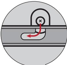
8. Once all nailheads are lined up in their respective rail slots, lower the Platform so equipment is fully supported by the rails. Reverse these steps for un-racking server equipment.
