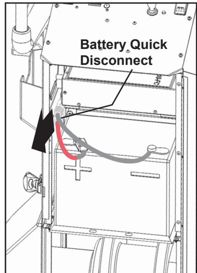
ⓘ **Note:** *Remove with care – Batteries weight 52 lb (23.5 kg)*
