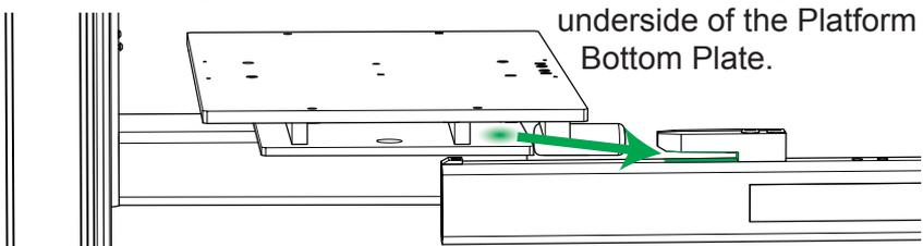
4. Ensure Rear Latch Tabs are fully engaged on the Platform as shown.
