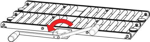
Rotate the handle counter-clockwise to unlock.
