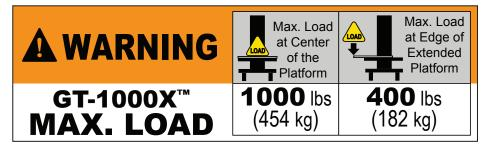
Max. load rating is ALWAYS superceded by ServerLIFT unit load rating.
